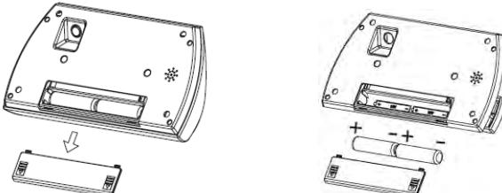
Insert the new batteries with the "+" side pointing as in the drawing
