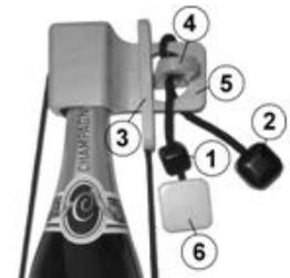
2) Push block "6" through the slot of of bar "4".
