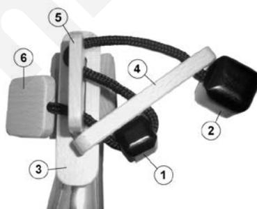
5) Now it should look like this. Push the cube "1" through the hole of bar "5", then slide bar "4" off the end of bar "5". Pull bar "3" towards you to set the bottle free.
