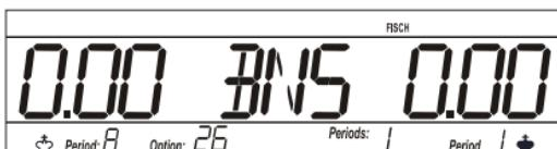
The next step would be to set the bonus time per move. With the  $+$  or  $-$  button you can change each digit separately. Then you can accept the value and go to the next digit with the  $\blacktriangleright$  button.
