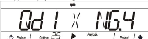
When there is a connection with a computer the  $\rightleftharpoons$  symbol will be shown in the top of the display.
