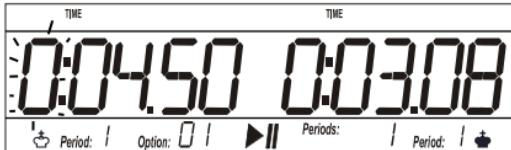
With the + or - button the value of the blinking digit can be changed. As soon as it has the desired value, you can select the next digit with the ► button. This digit starts blinking and can be changed. Continue doing this until all digits are set correctly. After accepting the far right (10<sup>th</sup>) digit the display will change and display the number of moves.
