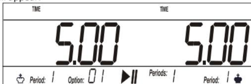
At this moment the position of the lever determines which side of the clock will count down first. The side on which the lever is up will start first. This will be indicated with the white ♚ icon at that side of the display. On the other side the black ♚ icon will be shown.
